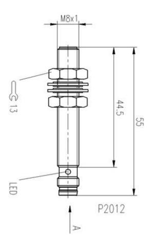
Inductive Sensors BES 516-378-S49-C M8x1 x 55 normally-closed Sn=1,5mm shielded
